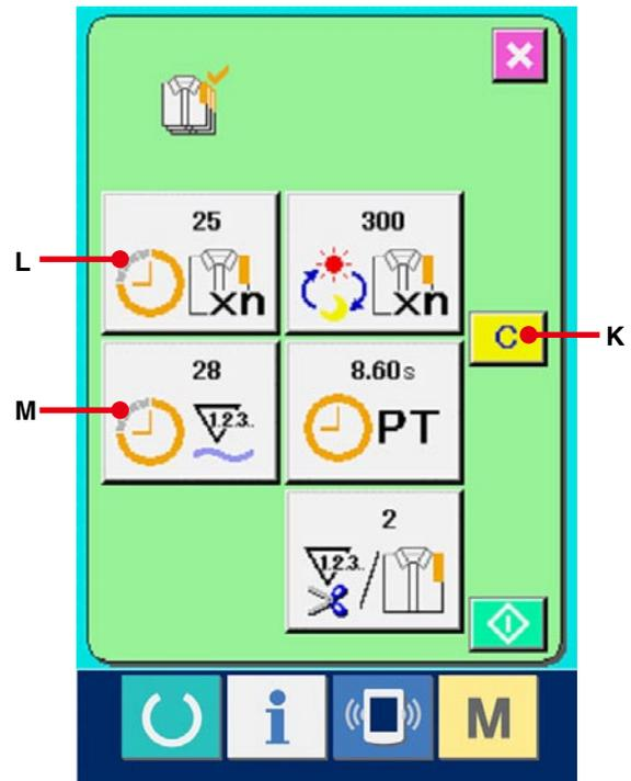
When CLEAR button **C** (N) is pressed in the clear confirmation screen. the counted value is cleared.
