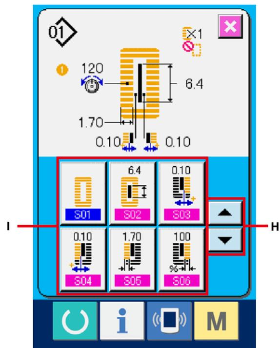
※ Now, input has been completed. However, for the continuous stitching, enter all data within the range of the presser size. When the data is outside the range, error is displayed. Be sure to correctly input the presser size.
