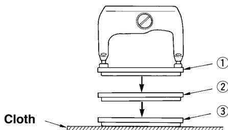
※ Height of the respective positions of ① to ③ described on the left side can be set or changed by the memory switches.
