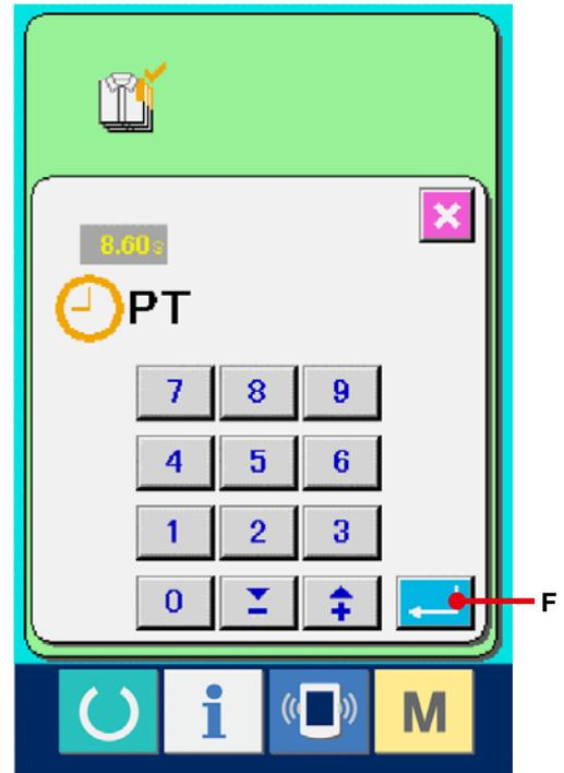
④ **Input the number of times of thread trimming.**
