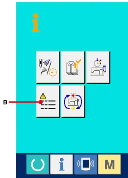
Error record of the sewing machine you use is displayed in the error record screen, and you can check the error.
