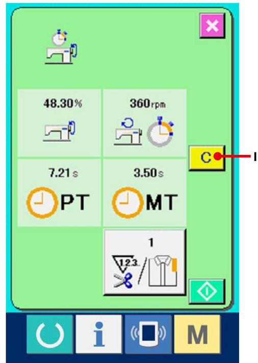
When CLEAR button **C** (J) is pressed in the clear confirmation screen, the counted value is cleared.
