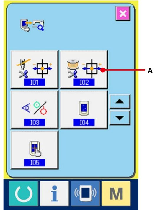
② **Perform the bobbin thread trimmer origin adjustment.**
