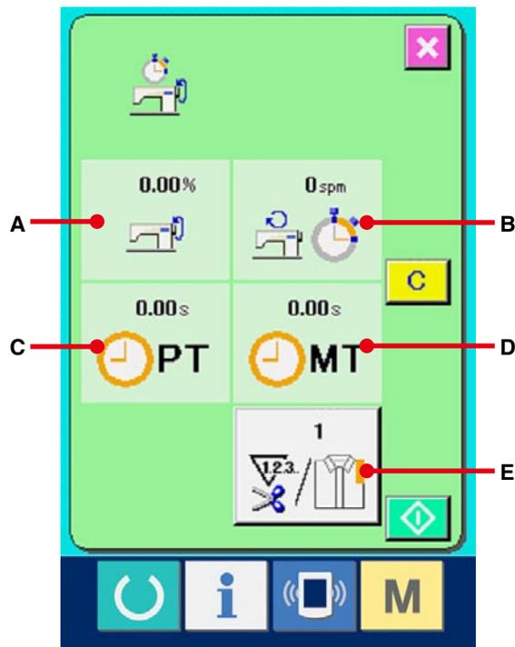
③ **Input the number of times of thread trimming.**
